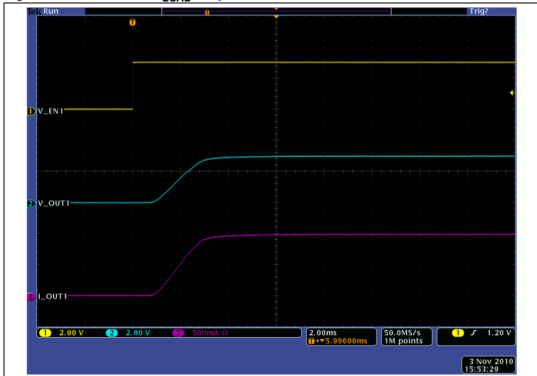
Figure 23. Turn-on for C_{LOAD} = 1\ \mu\text{F}
