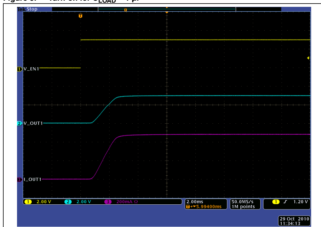
Figure 3. Turn-on for C_{\text{LOAD}} = 1\ \mu\text{F}
