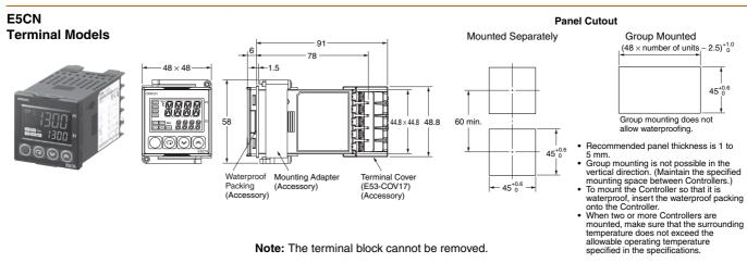
Note: The terminal block cannot be removed.
