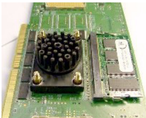
Figure 7-13. Allen screws removed
