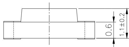
For reflow soldering (propose)
