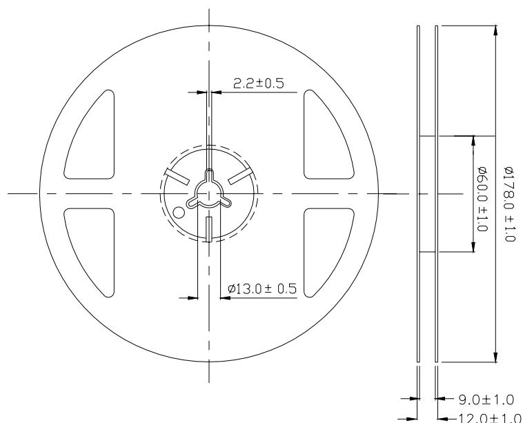
**Note:** The tolerances unless mentioned is  $\pm 0.1$  mm ,Unit = mm**Carrier Tape Dimensions: Loaded quantity 2000 PCS per reel**
