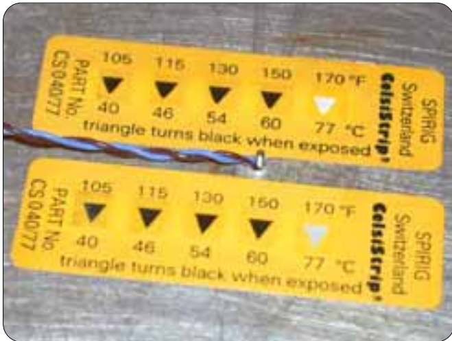
CelsiStrip® with 5 temperature levels. Also 8 levels (not shown here) available. Here 60°C are exceeded but 77°C never reached.
