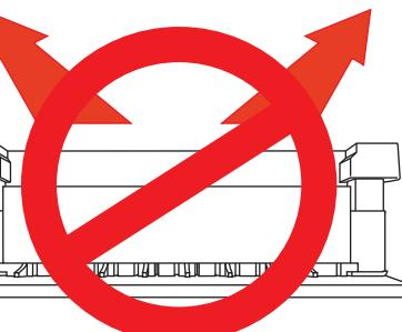
Pull the actuator as horizontally as possible by a proper force
