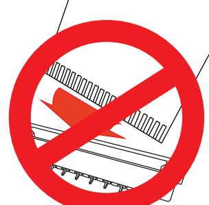
Do not keep FFC inclined when insertion
