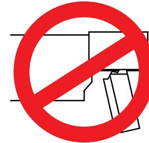
Do not pull the actuator too far otherwise the stop limit (hook on actuator) may be broken
