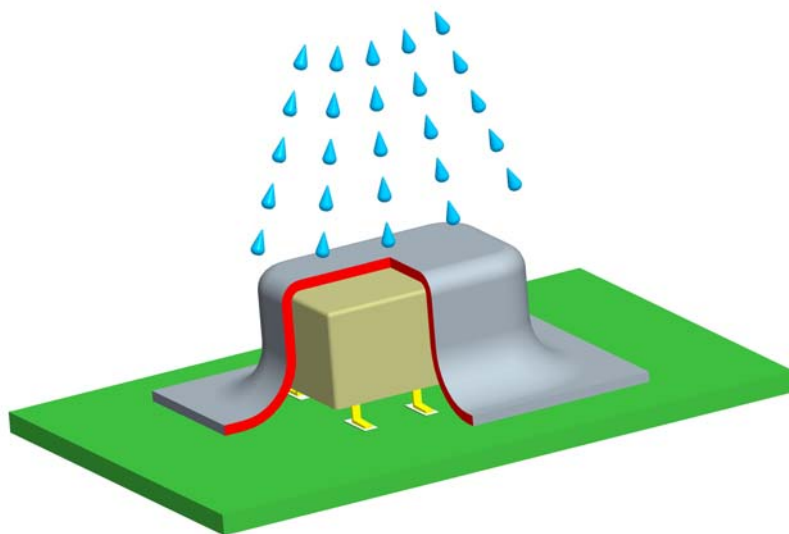
Fig. 11: Coating of relays on PCB's
