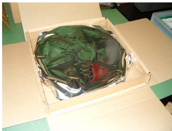
Fig. 3: "Pizza Box" for protection of the relays. Opened box with shock absorbers on the right hand side
