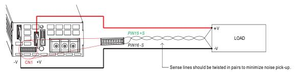
① The +S signal should be connected to the positive terminal of the load whereas -S signal to the negative terminal.
