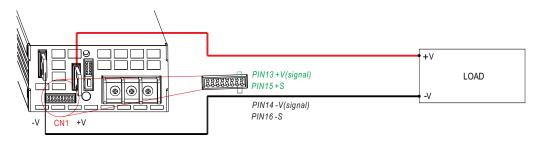
2. Output Voltage Programming (or, PV / remote voltage programming / remote adjust / margin programming / dynamic voltage trim)
