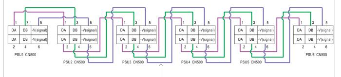
If the lines of CN500 are too long, they should be twisted in pairs to avoid the noise.
