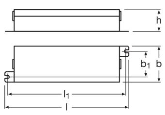
I = 170mm,  $I_1 = 163$ mm, b = 53mm,  $b_1 = 35$ mm, h = 38mm
