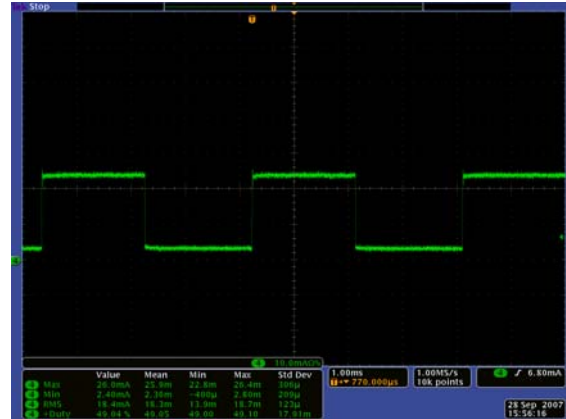
FIGURE 15. I_{LED} AT 50% PWM DIMMING
