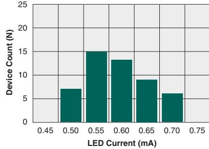
**Typical  $I_F$  for Switch Dropout
