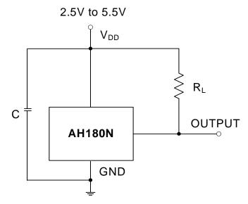
Note: C is for power stabilization and to strengthen the noise immunity, the recommended capacitance is  $10nF \sim 100nF$ .  $R_L$  is the pull-up resistor, the recommended resistance is  $10kOhm \sim 100kOhm$ .
