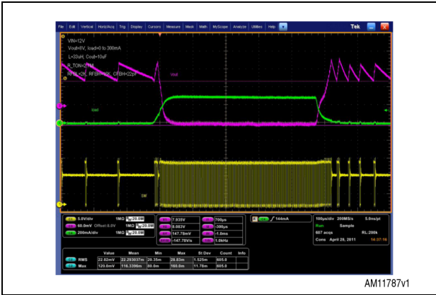
Figure 28. Load step = 0 to 300 mA
