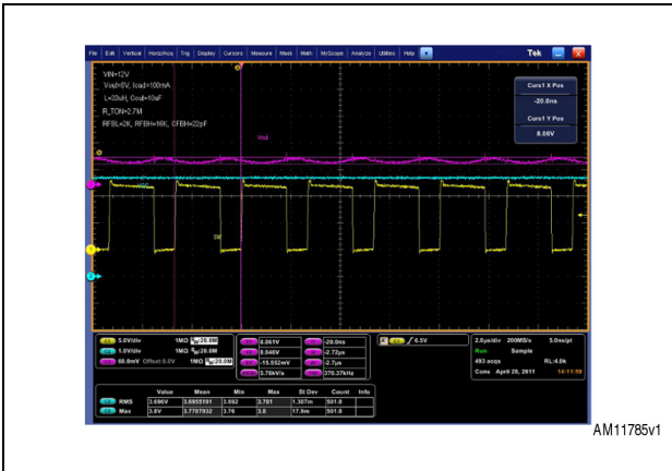
Figure 28. Load step = 0 to 300 mA
