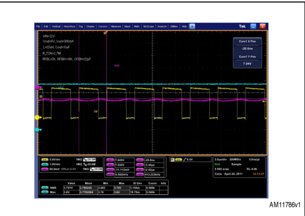
Figure 27. Load = 300 mA. Switching frequency = 410 kHz
