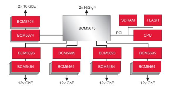
The BCM5674 10-Gigabit Ethernet switch is a scalable, multilayer switch-on-chip member of the StrataXGS family. The BCM5674 is a dual-port switch, which supports a 10 Gigabit Ethernet (IEEE 802.3ae) port and a HiGig<sup>™</sup> uplink port. The 10 Gigabit Ethernet port can be used to interface to the XENPAK module via the XAUI interface.
