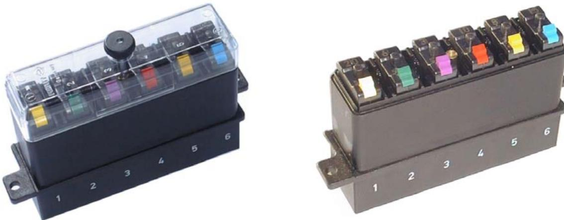
This base for the 1170 type circuit breaker will accommodate up to 6 circuit breakers of the same or mixed amperage ratings. The range is available from 3 amps to 30 amps and the amperage rating is etched on top of each circuit breaker. Each rating is also identified with an industry standard colour coded manual release trip lever.
