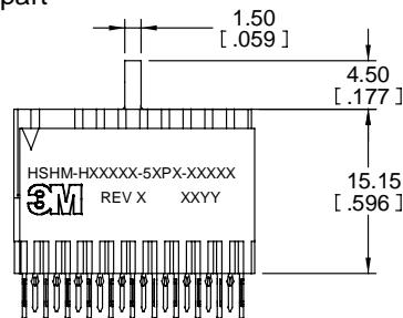
Coaxial, column differential and stripline configuration shown with protective caps\*
