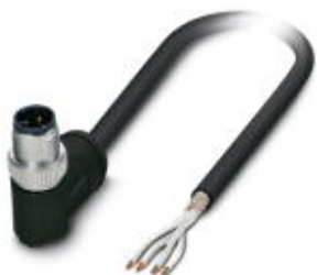
Sensor/actuator cable, 4-position, PE-X halogen-free, black, shielded, Plug angled M12 SPEEDCON, A-coded, on free cable end, cable length: 5 m, For railway applications
