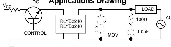
**Note:** Under certain low power factor load conditions, it may be advisable to connect an RC snubber network across the relay output. A snubber is also useful in the event of severe high voltage line spikes. While these do not generally cause damage to the relay, they may induce false cycle turn-on.
