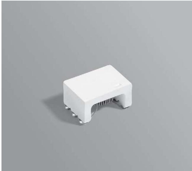
This low cost transformer is designed for use at 50 kHz to 300 kHz to sense continuous currents up to 3 Amps. The current windings can be connected in series to provide twice the output sensitivity. It is packaged in a small footprint, low profile, surface mount ceramic case that makes it ideal for pick and place operations.
