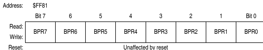
Figure 2-8. FLASH-2 Block Protect Register (FL2BPR)
