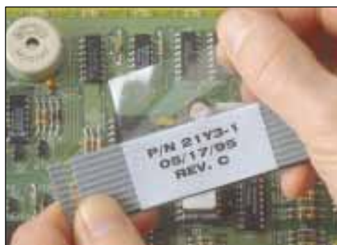
Flat Ribbon Cable Labeling
