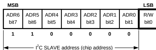
Figure 41. I 2 C Chip Address (see note above)
