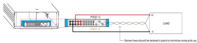
① The +S signal should be connected to the positive terminal of the load whereas -S signal to the negative terminal.
