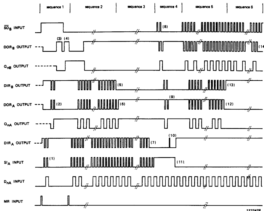
Fig.22 Waveforms showing the functionally and inter-communication between two FIFOs (refer to Fig.19).
