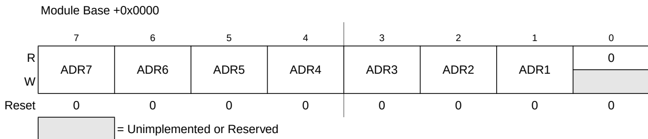
Figure 10-3. IIC Bus Address Register (IBAD)
