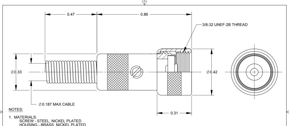
SCREW - STEEL, NICKEL PLATED HOUSING - BRASS, NICKEL PLATED SPRING - STEEL, NICKEL PLATED WASHER - PHENOLIC EYELET - BRASS, TIN PLATED COUPLING RING - NICKEL PLATED
