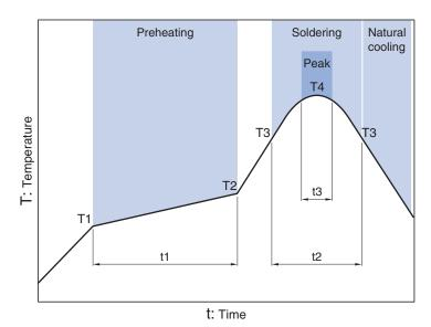
Soldering Preheating Peak Temp. Time Temp. Time Temp. Time T1 T2 T4 Т3 t2 t3 t1 150°C 180°C 60 to 120s 230°C 10 to 30s 245°C 5s
