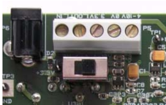
Figure 4: Power switch setting
