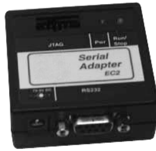
Figure 2: EC2 serial adapter
