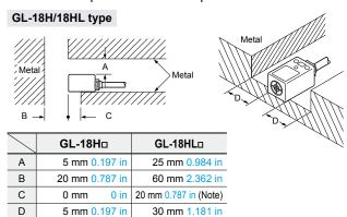
Note: When mounting the GL-18HL to an insulator or using the attached sensor mounting bracket, "C" becomes 0 mm 0 in.
