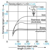
As the sensing object size becomes smaller than the standard size (iron sheet 25 × 25 × t 1 mm  $0.984 \times 0.984 \times t \ 0.039$  in), the sensing range shortens as shown in the left figure.
