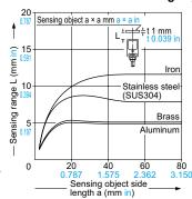
As the sensing object size becomes smaller than the standard size (iron sheet 40 × 40 × t 1 mm  $1.575 \times 1.575 \times t \ 0.039$  in), the sensing range shortens as shown in the left figure.
