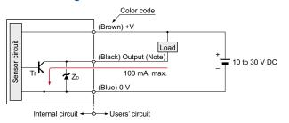
Note: Please carry out the wiring carefully since protection circuit against reverse power supply connection is not incorporated. Further, the output does not incorporate a short-circuit protection circuit. Do not connect it directly to a power supply or a capacitive load.
