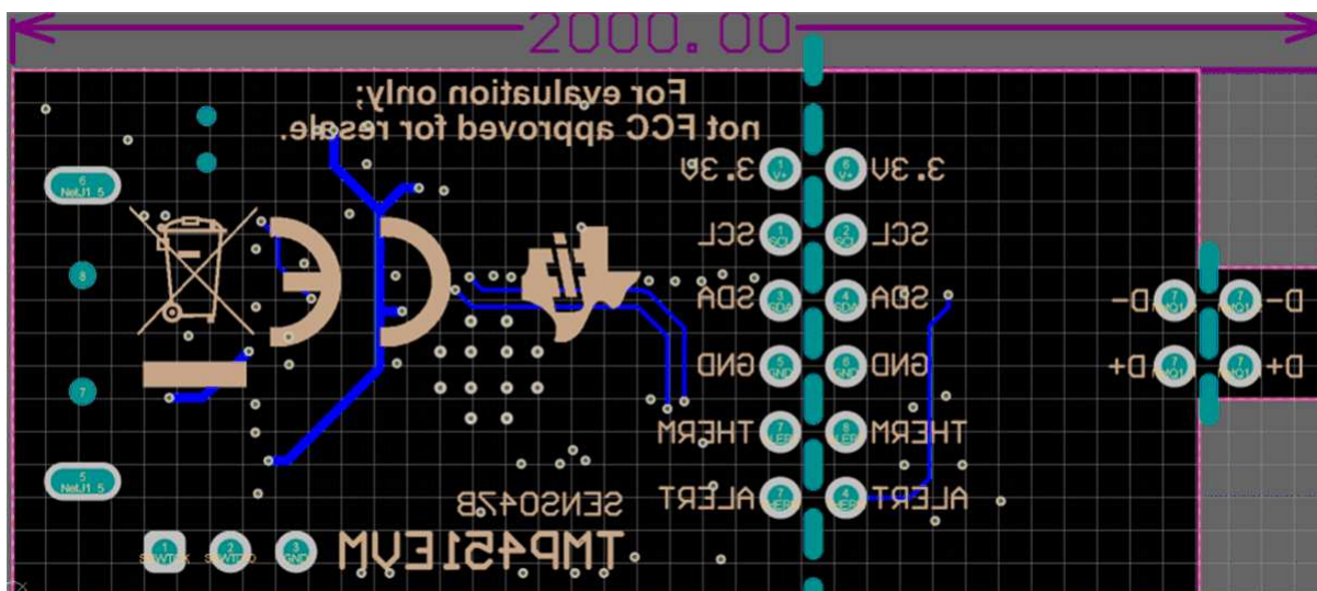
Figure 4-7. Bottom Assembly Layer
