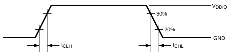
Figure 10. Deserializer LVCMOS Transition Times
