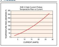
IDI current ratings are defined as the maximum current at which the temperature rise of the probe does not exceed 144°F (80°C) for a single probe in free air at ambient temperature for one hour
