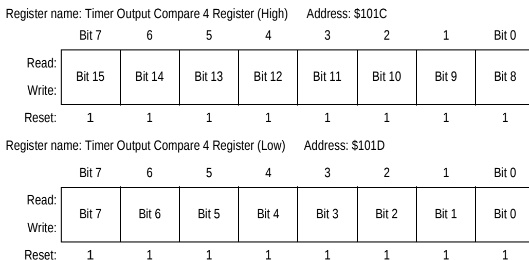
Figure 9-11. Timer Output Compare 4 Register Pair (TOC4)
