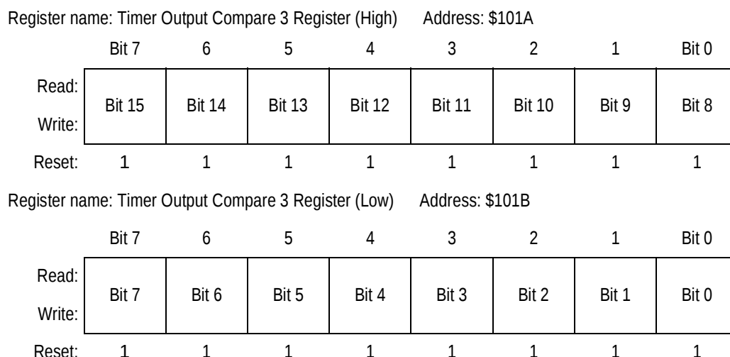
Figure 9-10. Timer Output Compare 3 Register Pair (TOC3)
