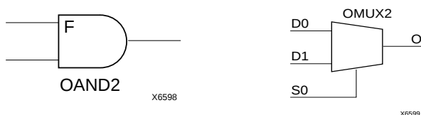
Figure 20: AND & MUX Symbols in XC4000X IOB
