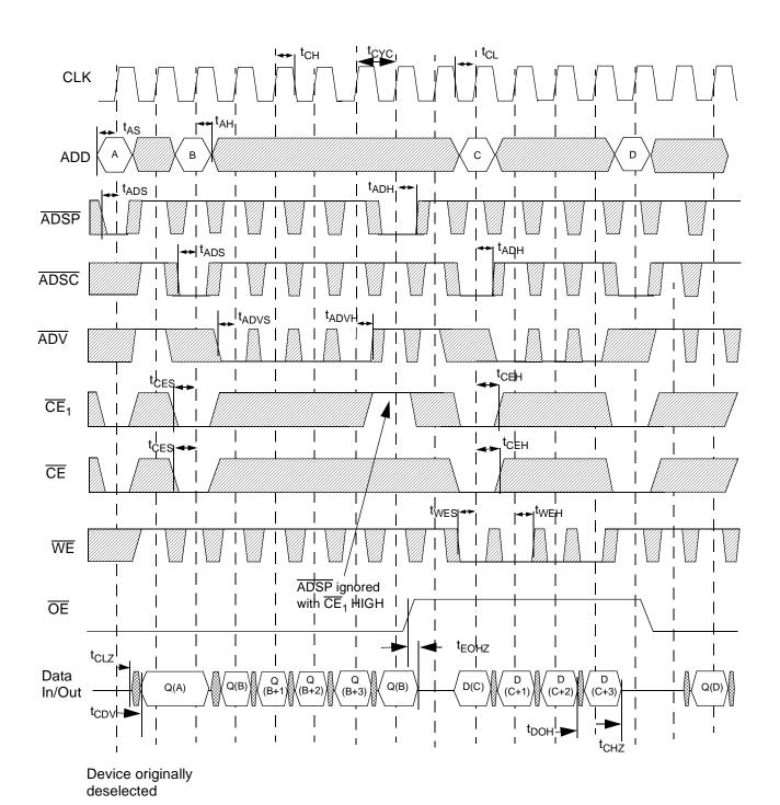
$\overline{\text{WE}}$  is the combination of  $\overline{\text{BWE}}$ ,  $\overline{\text{BWS}}_{[1:0]}$ , and  $\overline{\text{GW}}$  to define a write cycle (see Write Cycle Descriptions table).  $\overline{\text{CE}}$  is the combination of  $\text{CE}_2$  and  $\overline{\text{CE}}_3$ . All chip selects need to be active in order to select the device. RAx stands for Read Address X, WAx stands for Write Address X, Dx stands for Data-in X, Qx stands for Data-out X.
