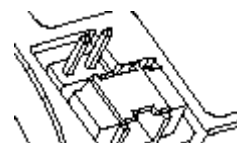
Figure 9: Master Setting for Vertical iDiskOnChip 40-Pin Connector
