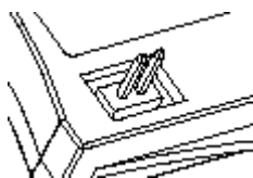
Figure 8: Master Setting for Vertical iDiskOnChip 44-Pin Connector
