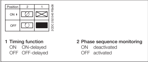
DIP switch functions CM-MPS.x1
