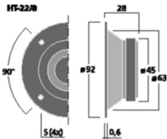
**Cone tweeter, 20WMAX, 8 Ohm** Classic tweeter for general applications in hi-fi, car hi-fi and for replacement purposes. **Klang+Ton 02/2012** "The unit at the most favourable price was the surprise in the test ... provides the most balanced frequency response in front of the microphone ... very attractive price, to be used without any problems, offers best measured values."
