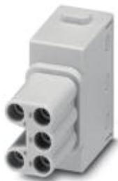
Contact insert module, number of positions: 5, power contacts: 5, control contacts: 0, Socket, Push-in connection, 400 V, 16 A, 0.14 mm<sup>2</sup> ... 2.5 mm<sup>2</sup>, application: Power
