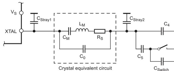
Using  $C_4 = 9.2pF \pm 2\%$ ,  $C_5 = 6.8pF \pm 5\%$ , a switch port with  $C_{Switch} = 3pF \pm 10\%$ , stray capacitances on each side of the crystal of  $C_{Stray1} = C_{Stray2} = 1pF \pm 10\%$ , a parallel capacitance of the crystal of  $C_0 = 3.2pF \pm 10\%$  and a crystal with  $C_M = 13fF \pm 10\%$ , typically results in an FSK deviation of  $\pm 21.5kHz$  with worst case tolerances of  $\pm 16.8kHz$  to  $\pm 28.0kHz$ .
