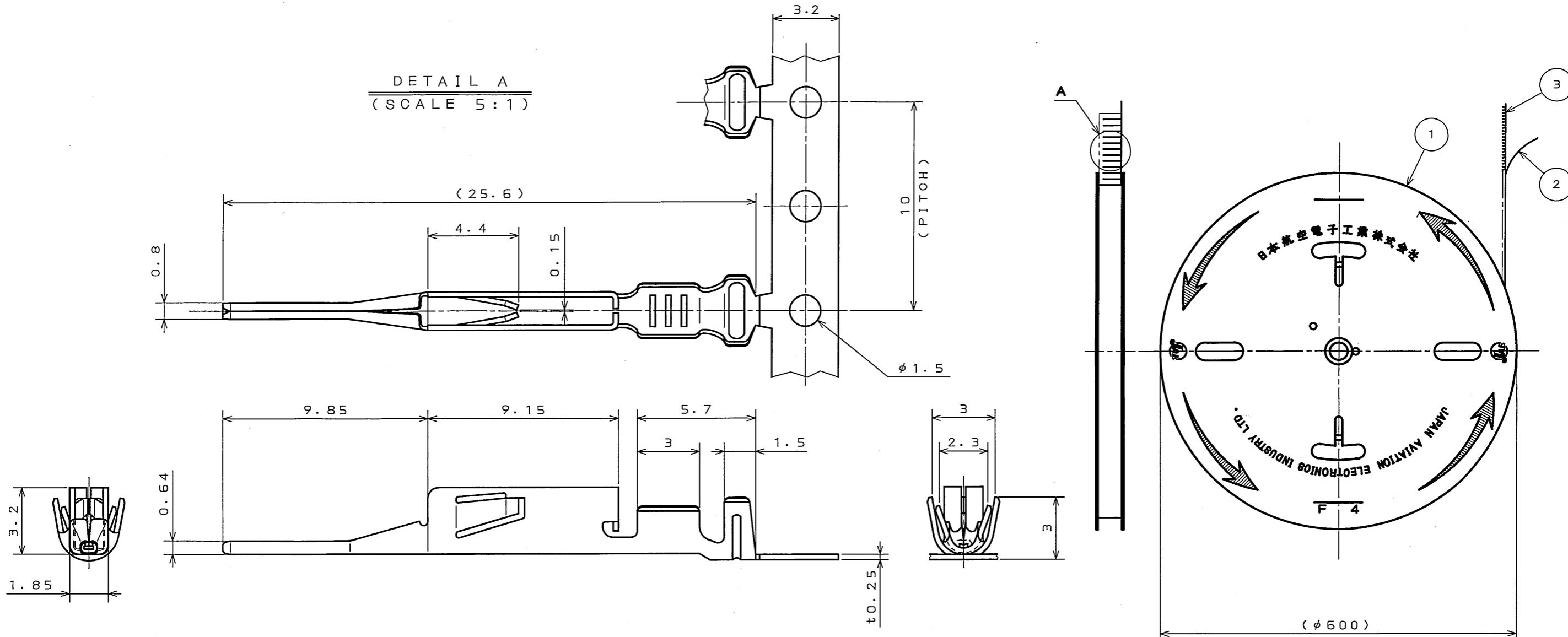
NOTE1. APPLICABLE WIRES SHALL BE AWG#22 TO #18(0.33 TO 0.82mm<sup>2</sup>)
