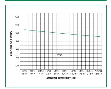
Note: 1. Derating depicted in this curve is in addition to the standard derating of 25% for  $\,$
