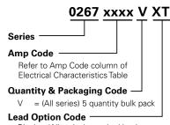
Blank = (All series) standard lead XT = (267 series only) solder coated lead option
