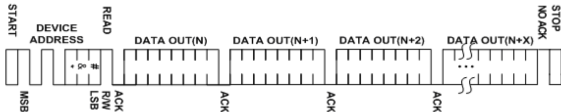
Figure 7: SEQUENTIAL READ (SDA INPUT/OUTPUT)
