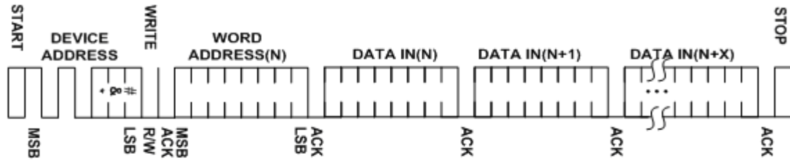
Figure 4: PAGE WRITE INSTURCTION (SDA INPUT)
