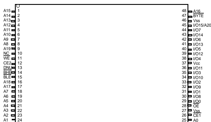
Figure 2. 48-pin TSOP I pinout (Top View) [4]
