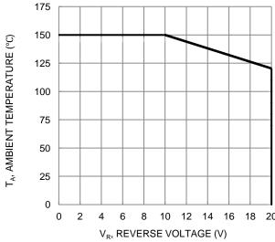
Figure 4. Operating Temperature Derating
