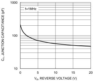
Figure 3. Typical Junction Capacitance
