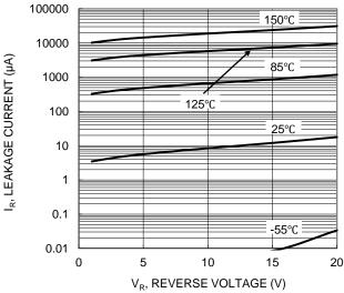
$V_{\rm R}$ , REVERSE VOLTAGE (V) Figure 2. Typical Reverse Characteristics
