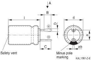
The series B41898 has no sleeve nor minus pole marking, the positive pole is marked on the aluminum case side instead.
