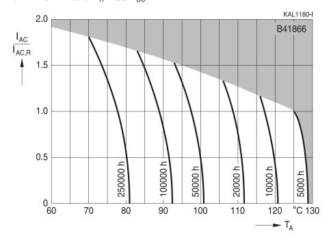
Useful life¹) depending on ambient temperature  $T_A$  under ripple current operating conditions  $V_R = 75 \ V_{DC}$
