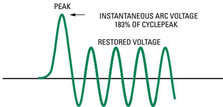
Figure 12 – Transient overvoltage during arcing time
