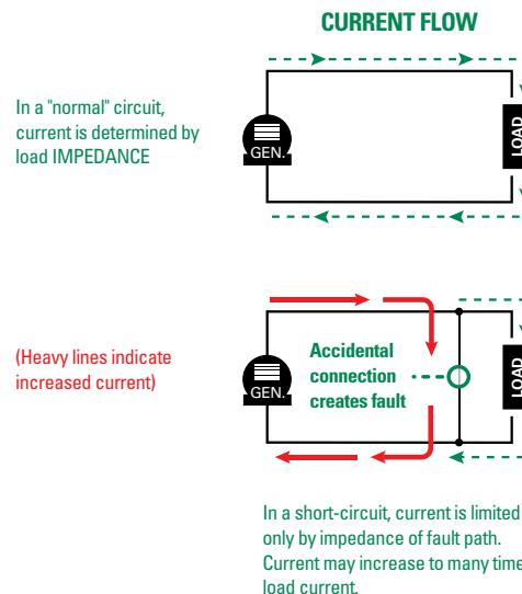
Figure 16 – Current Flow in Normal and Short Circuit Situations
