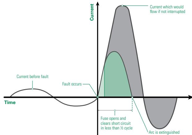
Figure 13 – Current-limiting Fuse
