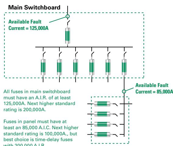
Figure 1 – Interrupting Rating Requirements per NEC
