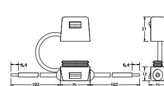
Used with ATO Fuse 1 to 20 A or 25 A and 30 A. Supplied with two 4" (102mm) wire leads. Includes protective cover for harsh environments.
