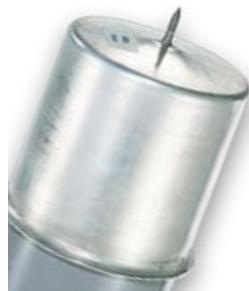
Current-limiting E- and R-rated fuses are equipped with a mechanical indicator or striker pin that protrudes through the fuse cap upon operation of the fuse. This provides visual identification of a blown fuse and can be used as a trigger for external devices.
