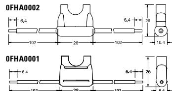
Used with ATO Fuse 1 to 20 A or 25 A and 30 A. Supplied with two 4" (102mm) wire leads.
