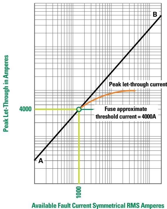
Figure 19 – Determining Threshold Current from Peak Let-through Chart
