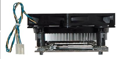
The Systium® Model 10312-25 heatsink was created for both socket 775 and 1155/1156 making CPU transitions easier. This low profile is only 35mm high but comes with a solid copper core allows it to cool processors up to 65W. Most heatsinks have the fan fixed permanently to the extrusion but this fan is easily replaced.
