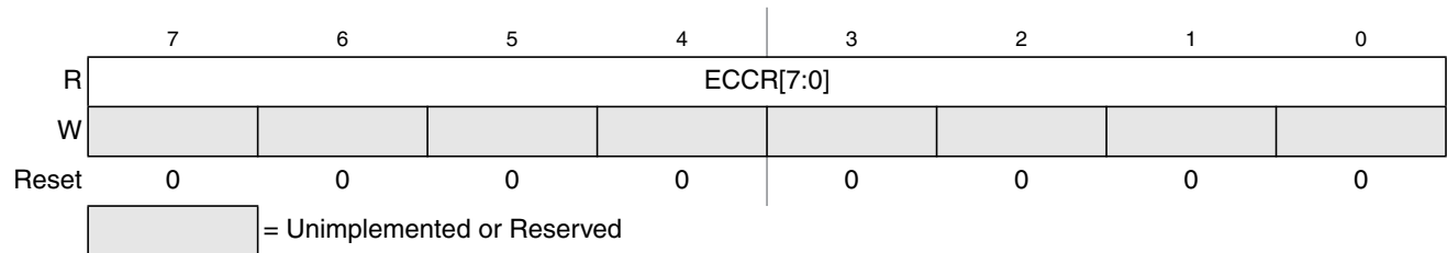
Figure 27-21. Flash ECC Error Results Low Register (FECCRLO)
