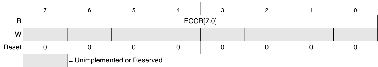
Figure 28-21. Flash ECC Error Results Low Register (FECCRLO)
