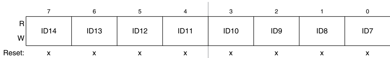
Figure 16-28. Identifier Register 2 (IDR2) — Extended Identifier Mapping
