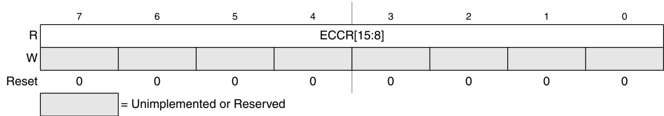
Figure 28-20. Flash ECC Error Results High Register (FECCRHI)
