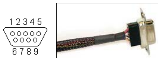
Figure 3: DB-9 Female Cable Connector (Rear View)
